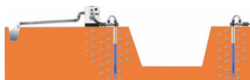
Active drainage by well point system
